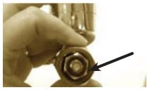
$\begin{array}{l} \textbf{STEP 1} \\ \textbf{High pressure washer installed into CO}_2 \\ \textbf{regulator (may already be installed)}. \end{array}$
